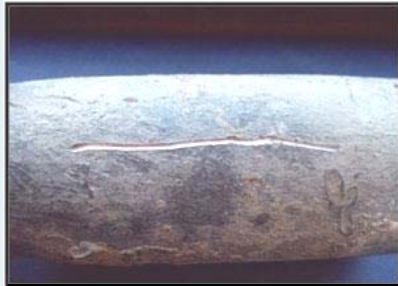
Lead pipe scratched with a key (photo courtesy of US EPA Region 5)
